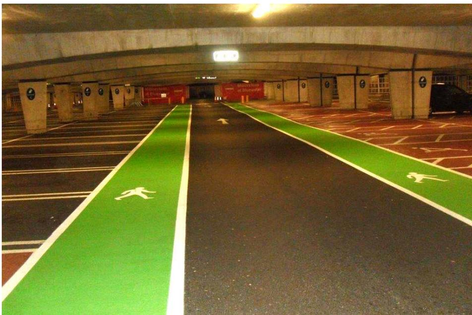
Pedestrian routes can be installed where space is available to do so, these routes should be segregated from vehicle routes if possible, they need to be clearly marked so drivers can identify them as a route for pedestrians, any areas where the route crosses a traffic lane should be marked with crossing panels.
